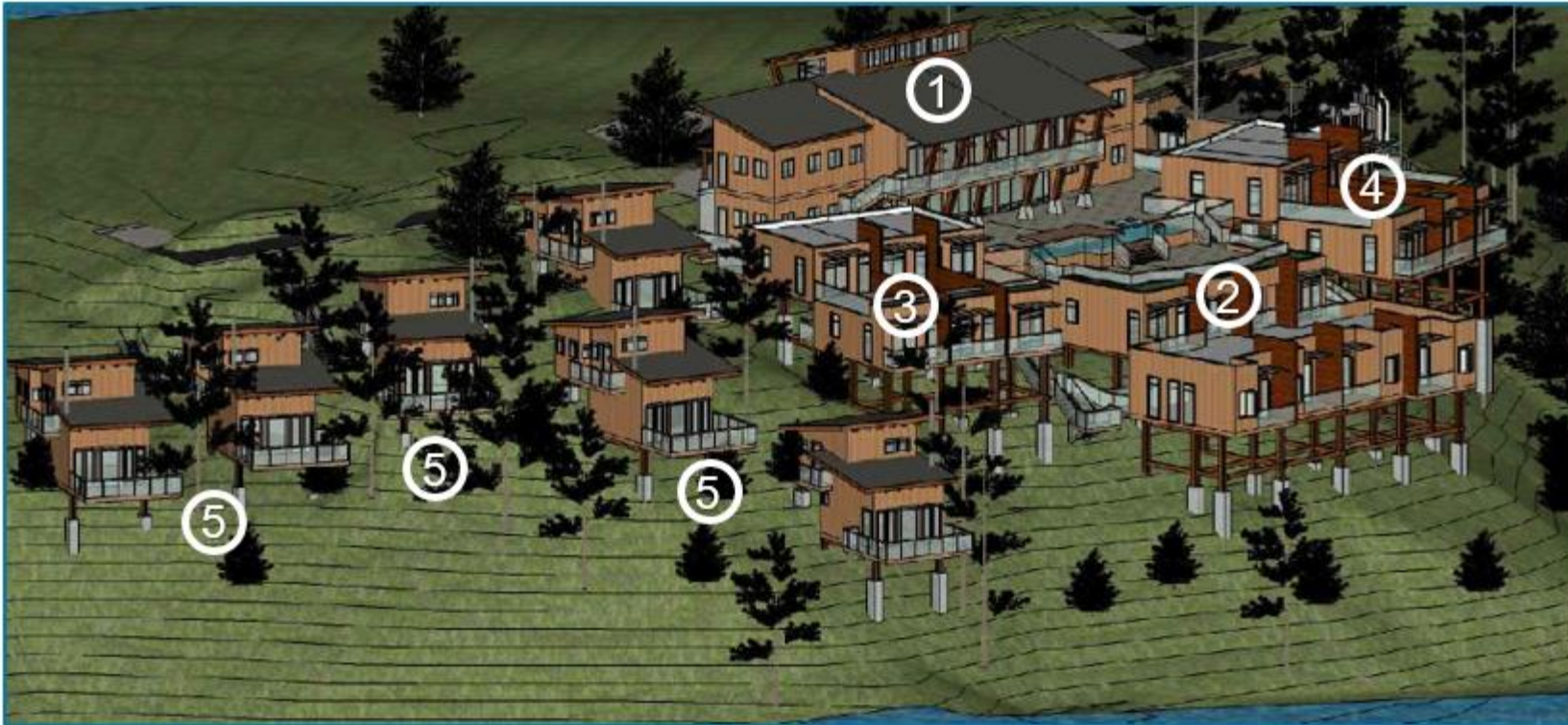
Figure 3. Project 3D render and footings. To minimize impacts associated with construction on the steep rocky slopes of the Subject Property , the main structures of the Proposed Development will be constructed over conventional concrete strips and pad/column footings. The image above shows a preliminary 3D render of the main hotel building (1), the hotel centre wing (2), the South (3) and North (4) wings, as well as the six duplex cabins (5). The Convention room, located behind the North wing is not visible from this perspective. Image modified from HNPA Architecture+Planning Inc. by Coastal Raintree Consulting, Ltd.
