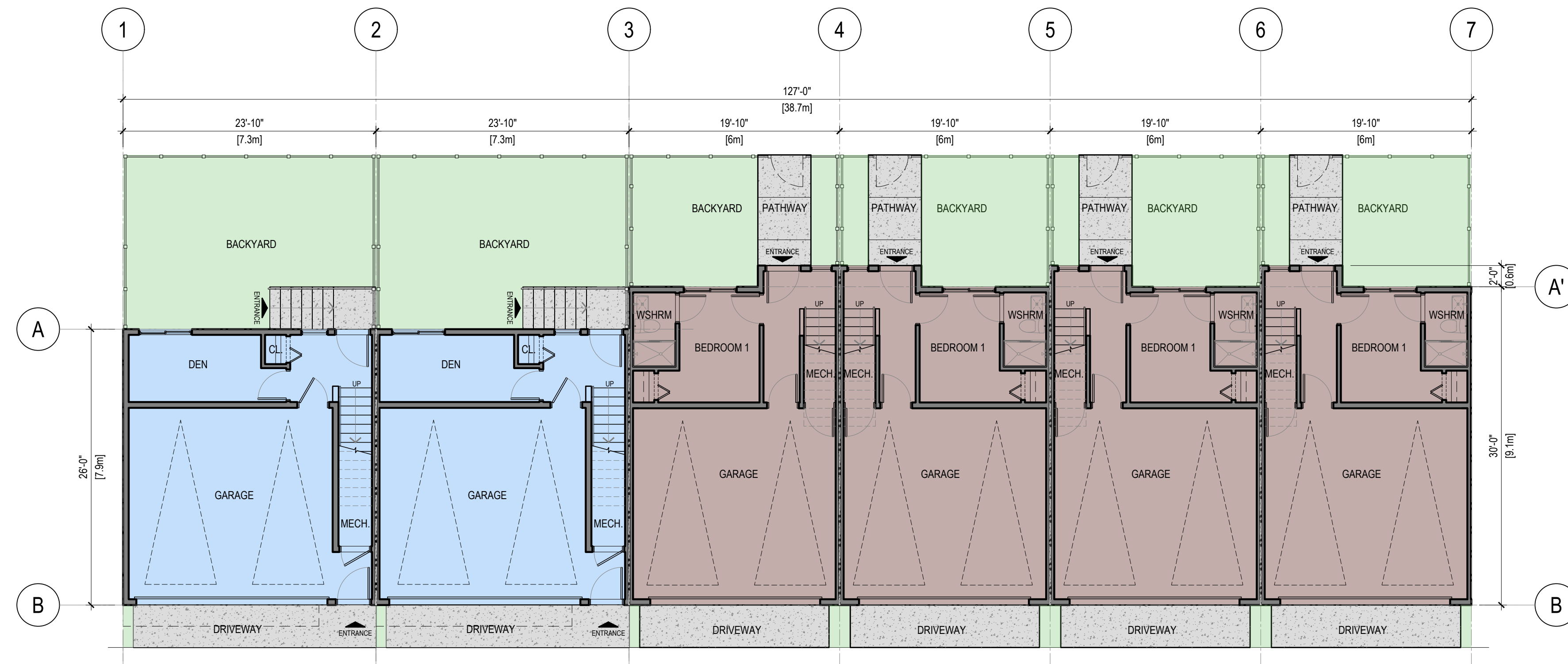
1 GROUND FLOOR PLAN - BUILDING 13 A2.11 SCALE: 1/8" = 1'-0"
