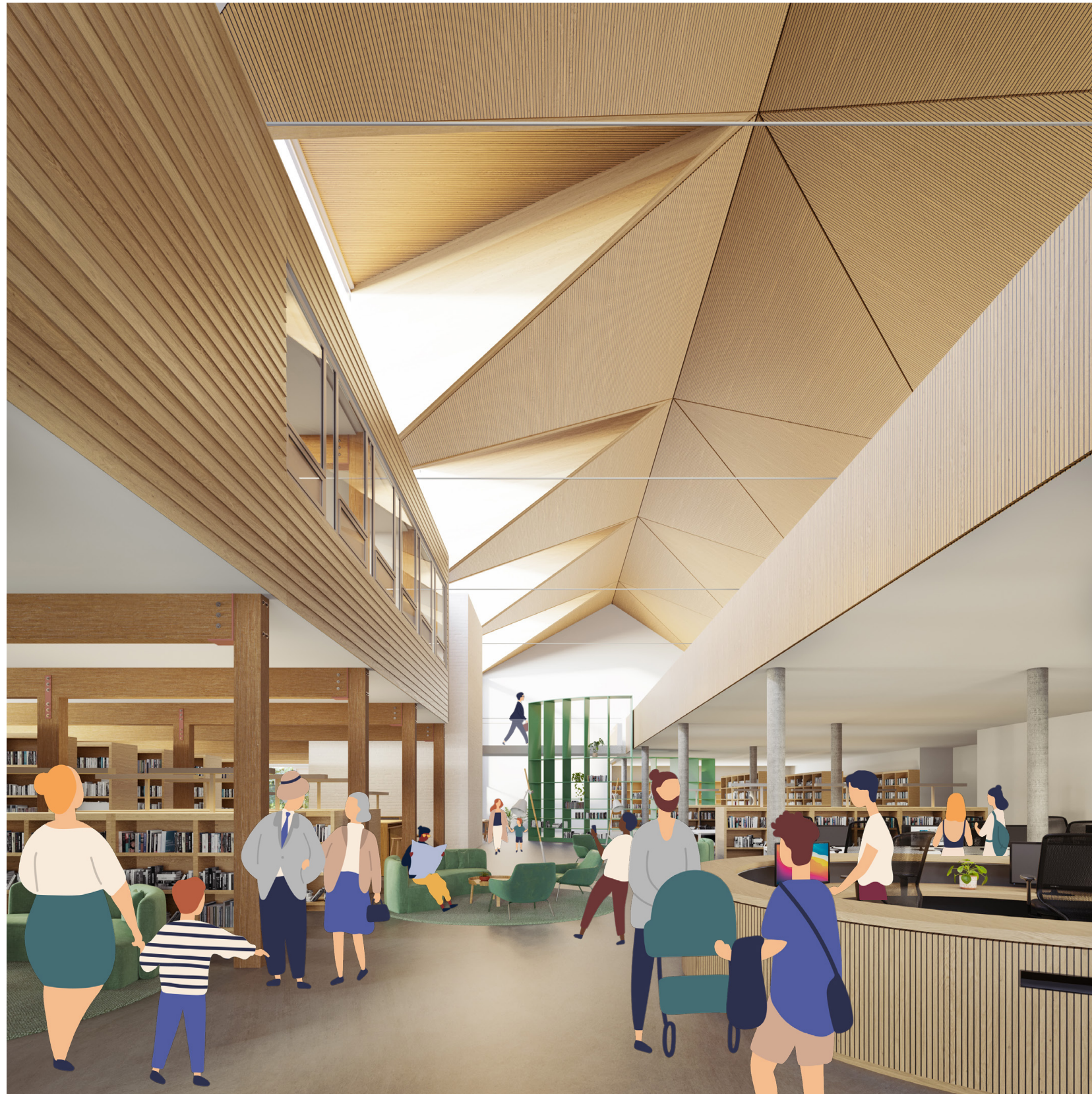
This concept ties the new building (right) addition to the exiting building (left) by creating a central atrium that delivers light to the center of the building for both the Library on the ground floor and the Municipal Hall upstairs. Illustrated by this artistic rendering above.
